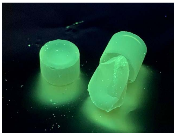
Fig. 1. Photoluminescence of aerogel-based luminescent material at an excitation wavelength of 380 nm
